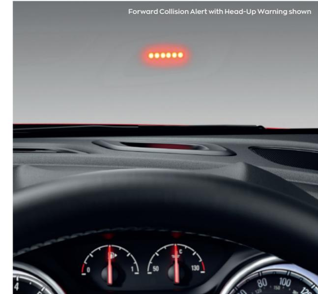
Forward Collision Alert with Head-Up Warning shown
