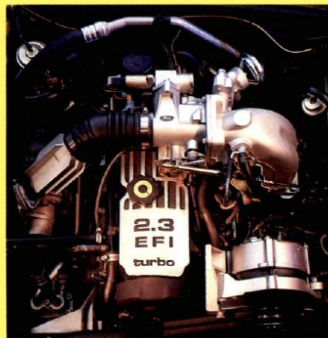
2.3-liter turbocharged OHC engine features advanced electronic controls.
