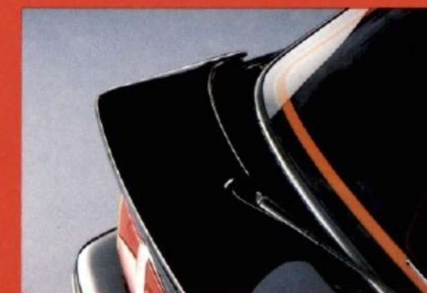
Decklid spoiler helps reduce rear-axle lift at speed.
