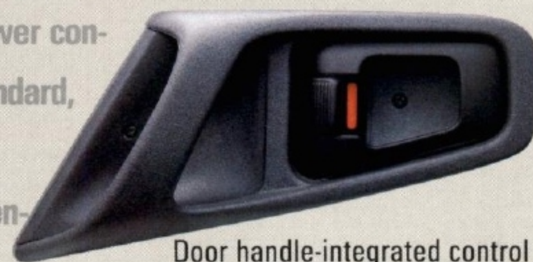
Door handle-integrated control for standard power door locks.
