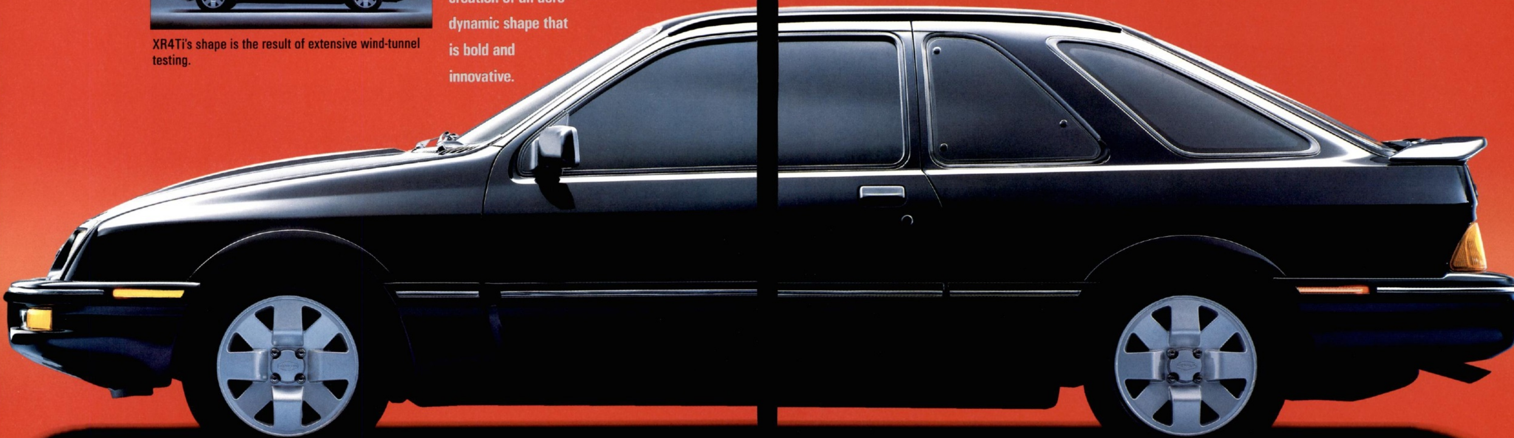
Decklid spoiler helps reduce rear-axle lift at speed.
