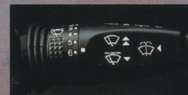
Control stalks adjust with steering column. stalks for the directionals, high beams and wipers/washer move along with it.
