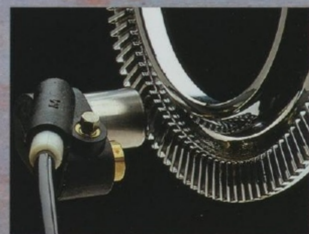
Sensors monitor wheel rotation and feed information to the ABS microprocessor.
