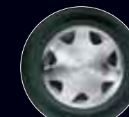
SLS Std.: 16" x 7" cast-aluminum wheels with Goodyear Integrity P235/60R16 S-rated tires
