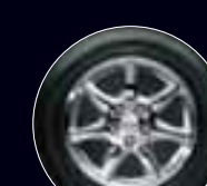
STS Opt.: 16" x 7" chromed cast-aluminum wheels STS Opt. Tire: Goodyear Eagle GA P235/60R16 Z-rated tires
