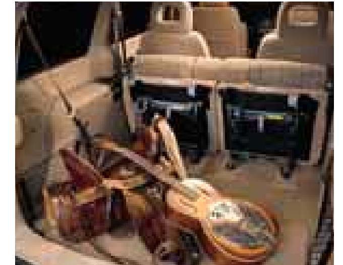
You can fold and stow the available rear seats for added space on demand. The seats can also be completely removed for even more cargo capacity.
