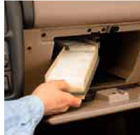
Trans Sport's not just capable of carrying a lot – it's even capable of improving your interior air quality. A changeable air quality filter helps reduce pollen and other irritants in the air.
