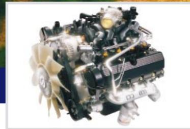
*The 5.4L V8 is one of the powerful Triton™ engines available with Econoline. Optional on the E-150 and standard on all E-350 models, its single-overhead-cam design is equipped with a maintenance-free silent chain drive which eliminates push rods and allows design flexibility for improved horsepower and torque.*
