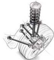
The multilink, double-wishbone rear suspension system adds excitement to spirited manoeuvres with crisp, confidence-inspiring handling.
