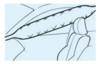
■ ITS Head Protection System (HPS) for the driver and front passenger provides effective protection of your head and upper body in a collision from the side.
