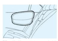
☐ Rear side airbags protect your upper body in a side-on collision: the side airbag significantly reduces the risk of injury at pelvic and chest level.
