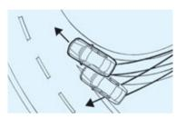
■ Dynamic Stability Control (DSC III) recognizes the risk of the car skidding very early and stabilizes the car within milliseconds. Also includes Dynamic Brake Control (DBC).
