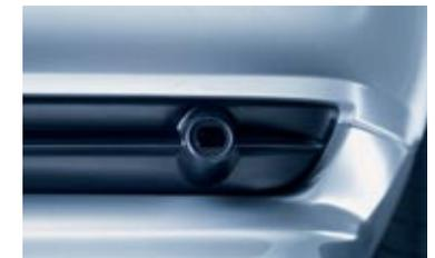
□ **Park Distance Control (PDC)** uses ultrasonic sensors in the rear bumper to help you judge the distance to other cars and unseen objects when parking. The beeping becomes faster as your bumper approaches the object, turning into a constant tone when the distance is less than 30 centimetres.
