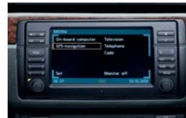
□ **On-board Navigation System** guides you conveniently and directly to your destination. In addition to providing driving instructions via voice, directional arrows or map display, the system will provide destination-specific information.
