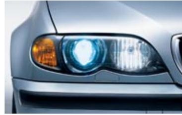
■ **Xenon headlights** (high and low beam) illuminate the road ahead and to the side with brilliant clarity. These headlights also feature auto-levelling to adjust for varying passenger and cargo loads. They also have twice the light intensity of conventional halogen bulbs.
