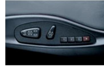
□ **Electric seats with driver memory** enable the driver and passenger to precisely adjust their seat to individual preferences. The positioning of the driver's power outside mirrors is also retained in the seat memory.
