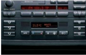
■ **Automatic climate control system** includes automatic air recirculation, which is activated when a sensor detects certain pollutants in the outside air. Inside, cabin air continuously passes through a microfilter that removes pollen, dust and spores.
