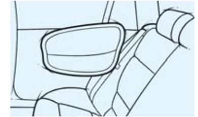
□ **Rear side airbags** protect your upper body in a side-on collision; the side airbag significantly reduces the risk of injury at pelvic and chest level.
