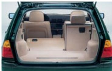
■ **Split-folding rear seats**, folding up and down in 2:1 split for variable layout of the luggage compartment when transporting bulky objects (bicycles, skis, etc).
