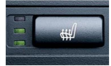
□ **Seat heating** is a welcome feature in cooler weather. With the touch of a button, you can individually select from three heat settings.
