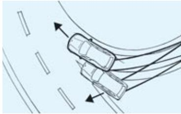
■ **Dynamic Stability Control (DSC III)** recognizes the risk of the car skidding very early and stabilizes the car within milliseconds. Also includes Dynamic Brake Control (DBC).
