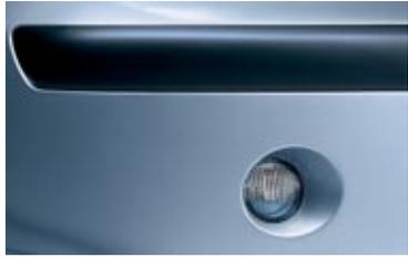
■ **Foglights** in free-form technology, integrated in the front air dam to give the driver better visibility and orientation in fog, snow and heavy rain. At the same time, the risk of dazzling from one's own lights is reduced.
