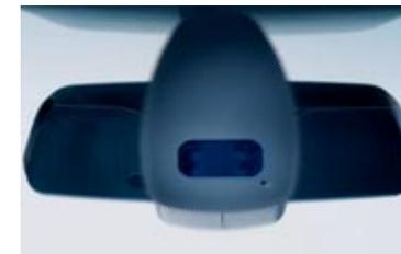
□ **Rain sensor** uses an infrared light to measure the amount of rain. When the wipers are in the "intermittent" mode, the rain sensor automatically adjusts the windshield wiping interval as needed. Also includes automatic headlamp function.
