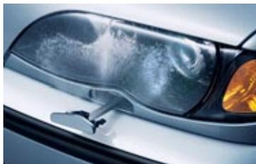
■ **Heated headlight washing system** helps keep lights clean of ice, mud, road salt and other coatings for maximum road lighting and enhanced driving safety.
