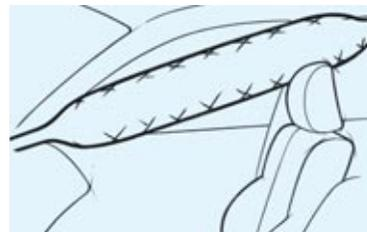
■ **ITS Head Protection System (HPS)** for the driver and front passenger provide effective protection of your head and upper body in a collision from the side.
