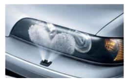
☐ Heated headlight washers help keep lights clean of ice, mud, road salt and other coatings, for maximum road lighting and enhanced driving safety. (Standard on 540iT.)
