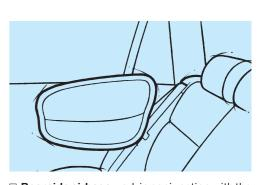
☐ Rearside airbags work in conjunction with the standard rear Head Protection System (HPS) to protect your upper body and head in a side-on collision; the side airbag significantly reduces the risk of injury at pelvic and chest level.
