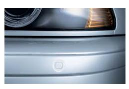
☐ Park Distance Control (PDC) uses ultrasonic sensors in the front and rear bumpers to help you judge the distance to other cars and unseen objects when parking. The beeping becomes faster as your bumper approaches the object, turning into a constant tone when the distance is less than 30 centimetres.
