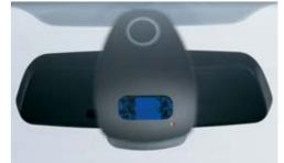
☐ Rain sensor uses an infrared light to measure the amount of rain. When the wipers are in the "intermittent" mode, the rain sensor automatically adjusts the windshield wiping interval as needed. (Standard on 540iT.)
