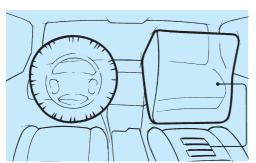
■ Driver and front passenger airbags protect your head and upper body in a frontal collision from hitting the steering wheel or instrument panel; depending on the severity of the impact, the airbags are inflated via a two-stage gas generator (impact-depending system); the front passenger airbag comes complete with a seat occupancy detector.
