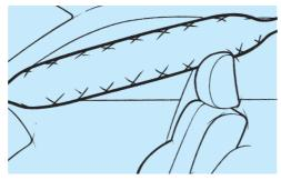
■ ITS Head Protection System (HPS) provides effective protection of both the head and upper body in the case of a side-on collision to both the front and rear passengers.
