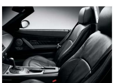
■ Sport seats for the driver and front passenger are designed to offer optimum lateral support in every driving situation. This is provided by highly-contoured seat bolsters and a wide range of settings, including individual adjustment for seat height and seat angle.
