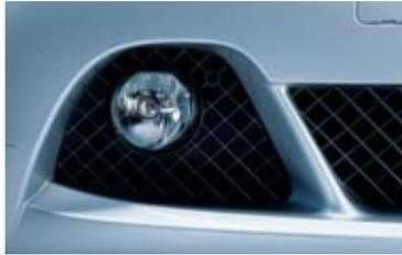
■ **Front bullet foglights** are cleanly integrated into the front bumper, illuminating the road ahead in poor weather.
