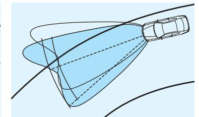
□ **Adaptive Headlights** allow the xenon headlights to actively adjust themselves to bends in the road and also light up the road ahead, offering significant improvement to road illumination, especially at night.
