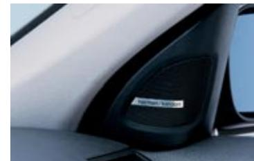
□ **Harman/Kardon Sound System** projects exceptional sound from upgraded speakers and amplification, plus a subwoofer and vehicle-speed-sensitive equalization.
