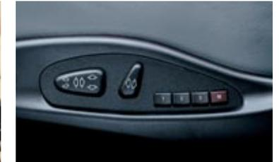
□ **Electric Seats with Driver Memory** enable the driver and passenger to precisely adjust their seats to individual preferences. The driver's mirror positioning is also retained in the seat memory.
