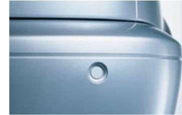
□ **Park Distance Control (PDC)** uses ultrasonic sensors in the rear bumper to help you judge the distance to other cars and unseen objects when parking. The beeping becomes faster as your bumper approaches the object, turning into a constant tone when the distance is less than 30 centimetres.
