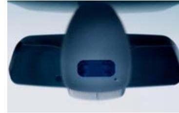
■ **Rain sensor** uses an infrared light to measure the amount of rain. When the wipers are in the "intermittent" mode, the rain sensor automatically adjusts the windshield wiping interval as needed. Includes automatic headlight function.
