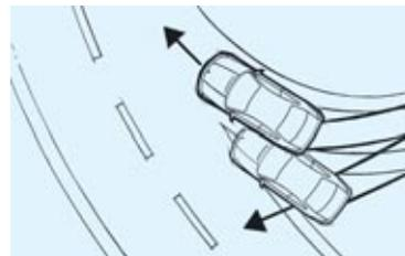
■ **Dynamic Stability Control (DSC)** recognizes the risk of the car skidding very early and stabilizes the car within milliseconds. Also includes Dynamic Brake Control (DBC).
