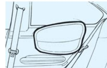
□ **Rear side airbags** protect your thorax in a side-on collision; the side airbag significantly reduces the risk of injury at pelvic and chest level.
