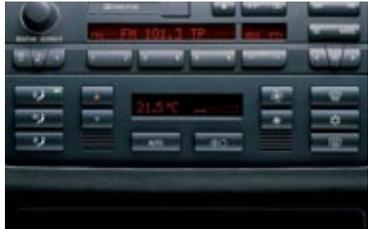
■ **Automatic Climate Control system** includes Automatic Air Recirculation (AAR), which is activated when a sensor detects certain pollutants in the outside air. Inside, cabin air continuously passes through a microfilter that removes pollen, dust and spores.
