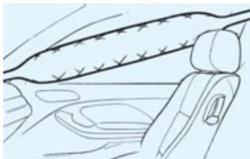
■ **Head Protection System (HPS)** for the driver and front passenger provides effective protection of your head and upper body in a collision from the side.
