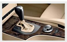
□ Six-speed automatic transmission with electronic gearshift and STEPTRONIC. You operate the transmission via the switch on the steering column or the STEPTRONIC buttons on the steering wheel. Electric shift-by-wire transmission allows a very quick and absolutely faultless shift of gears in the interest of supreme driving dynamics.
