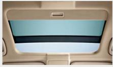
■ Glass sunroof allows natural light to enter the cabin. For convenience, it offers fingertip control of sliding and vent functions, trap release and comfort opening and closing.
