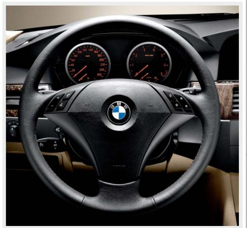
■ Multi-function leather steering wheel allows for convenient operation of numerous functions without being distracted from road traffic – which means you keep your hands on the wheel all the time. Buttons are included for audio, cruise control and telephone. One button's function may be defined by the user.
