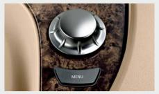
element for both the driver and the front passenger. This turn/press button enables intuitive control of a variety of functions shown on the Control Display. The menu system is based on the compass directions and provides a choice of four individually coloured menus: Climate, Navigation, Communication and Entertainment.
