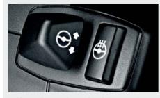
■ Heated steering wheel is a welcome pleasure whenever there is a chill in the air. The switch is conveniently located right on the steering column.
