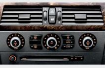
■ Automatic Climate Control including Automatic Air Recirculation (AAR) provides your desired climate as quickly as possible, keeping the temperature at a steady level separately on the driver's and front passenger's side.
