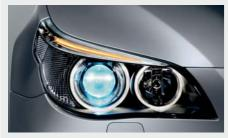
■ Xenon headlights illuminate the road ahead and to the side with brilliant clarity. These headlights also feature auto-levelling to adjust for varying passenger and cargo loads. In conjunction with the new Adaptive Headlights (optional), this also means much improved visibility in bends, as the adjustable headlights are directed into the bend as soon as the vehicle begins cornering.
