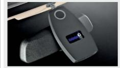
■ Rain sensor with automatic headlights uses an infrared light to measure the amount of rain and exterior light. When the wipers are in the "intermittent" mode, the rain sensor automatically adjusts the windshield wiping interval as needed. When selected, the xenon headlights are activated as required.
