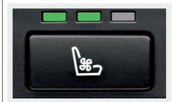
☐ **Ventilated seats** for the driver and front passenger. Ventilator fans are built into the outside seats and blow air upwards through an internal web and the micro-perforated Nasca leather to provide active ventilation.
