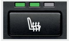
■ Heated seats, front and rear, are a welcome feature in cooler weather. With the touch of a button, you can individually select from three heat settings.
