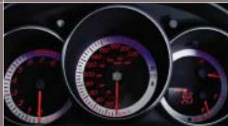
**GLOWING REPORT.** Tri-mode electro luminescent gauges, standard on the Mazda3 GT and Mazda3 Sport models, display three distinct colour combinations depending on whether it's daytime, night-time or the ignition is off.
