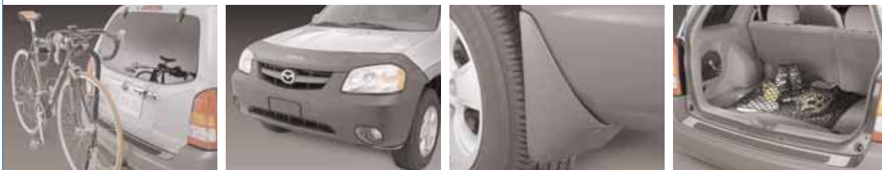
Pictured below from left to right: trailer-hitch bike attachment, front mask, rear mud guards and cargo net.
