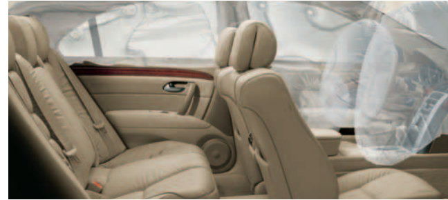
> Front, Side, and Side Curtain Airbags. Dual-stage, dual threshold front airbags are designed to deploy at two rates and thresholds, depending on severity of impact and seatbelt use. Side curtain airbags provide added protection.
