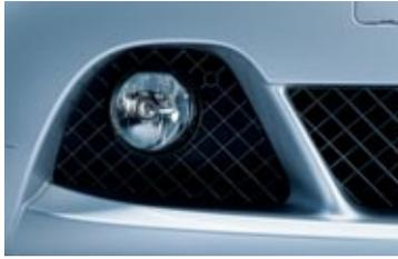
■ **Foglights** in halogen free-form technology are integrated into the front air dam, and ensure additional visibility and safety in bad weather or poor visibility.
