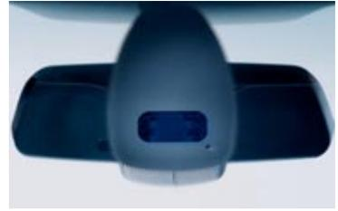
■ **The rain sensor** uses an infrared light to measure the amount of rain. When the wipers are in the "intermittent" mode, the rain sensor automatically adjusts the windshield wiping interval as needed. Includes automatic headlight function.
