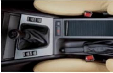
■ **Six-speed manual transmission** makes for extremely dynamic driving. Smooth and optimally synchronized, it boasts precise, short shift throws. The more tightly graded transmission and additional sixth gear make the engine even more responsive to your personal style of driving. (Available only on 330Ci.)
