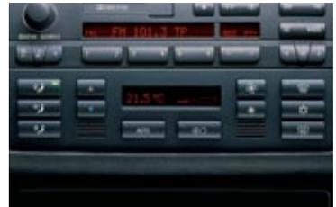
■ **Automatic Climate Control** includes Automatic Air Recirculation (AAR), which is activated when a sensor detects certain pollutants in the outside air. Inside, cabin air continuously passes through a microfilter that removes pollen, dust and spores.
