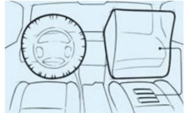
■ **Driver and front passenger airbags** protect your head and upper body in a frontal collision from hitting the steering wheel or instrument panel. Depending on the severity of the impact, the airbags are inflated via a two-stage gas generator (Impact-Dependent System); the front passenger airbag comes complete with a seat occupancy detector.
