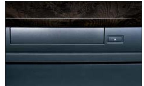
■ **CD changer** fitted above the glove compartment for easy and convenient use. Accommodates up to 6 CDs.
