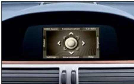
■ **Control Display** in LCD technology with screen. Using the Controller, you can present all functions masterminded by iDrive on the Control Display – for example, route information or other items such as the radio program or information from the on-board computer.
