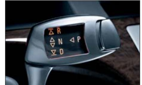
■ **Six-speed automatic transmission** with electronic gearshift and STEPTRONIC. You operate the transmission via the switch on the steering column or the STEPTRONIC buttons on the steering wheel. Electric shift-by-wire transmission allows a very quick and absolutely faultless shift of gears in the interest of supreme driving dynamics.
