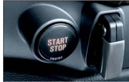
■ **Start/Stop button** for starting the car together with the remote control. Drivers insert the remote control into the starter switch until it rests in position. After receiving authorization, they can start/stop their BMW simply by pressing a button.
