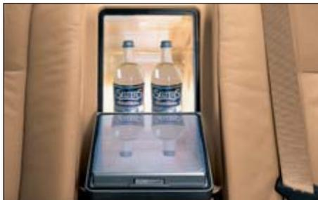
□ **Cooling box**, included with the rear air conditioning system, is accessible when the centre armrest is folded down, and provides capacity for one or two suitable drink bottles and some snacks. (Available only on the 745Li and 760Li.)
