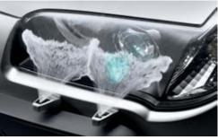
□ **Headlight washer system** provides automatic cleaning in parallel with the windshield wipers when the headlights are on, thereby enhancing the headlight illumination of the road ahead in all weather conditions.
