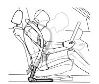
■ BMW restraint system for the driver and front passenger consists of a combination of the three-point seat belt, belt latch tensioner, belt force governor and anti-submarining ramp in the seat, for optimum restraint in a collision.
