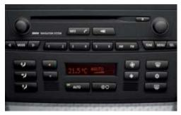
■ Automatic Climate Control system includes Automatic Air Recirculation (AAR), which is activated when a sensor detects certain pollutants in the outside air. Inside, cabin air continuously passes through a microfilter that removes pollen, dust and spores. (Optional on the X3 2.5i.)
