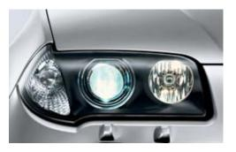
■ Xenon headlights for low and high beam, including dynamic headlight range control for much better illumination of the road ahead in bad weather or poor visibility. These headlights also feature auto-levelling to adjust for varying passenger and cargo loads.
