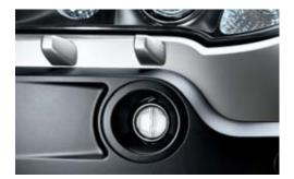
■ Foglights in halogen free-form technology are integrated into the front air dam, and ensure additional visibility and safety in bad weather or poor visibility.
