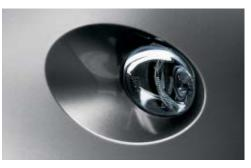
■ Foglights in halogen free-form technology are integrated into the front air dam to ensure additional visibility and safety in bad weather or poor visibility.
