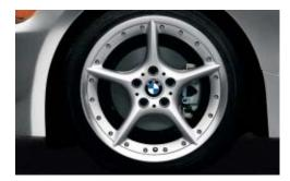
□ Star Spoke bolted wheels (with performance run-flat tires) - Style 108,  $18 \times 8.0$ , front, 225/40R-18;  $18 \times 8.5$ , rear, 255/35R-18. Tires not recommended for winter use. (Optional on Z4 3.0i.)
