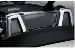
□ The **wind deflector** reduces drafts and isolated turbulence in the shoulder and neck region; consists of two panes securely fitted into the roll bars and a frame-based net spanning between them. If the net is not required, it can be stored in a special storage rack in the luggage compartment. Please see your local BMW Retailer for complete details.
