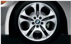
$\Box$  Ellipsoid alloy wheels (with performance run-flat tires) - Style 107, 18 x 8.0, front, 225/40R-18; 18 x 8.5, rear, 255/35R-18. Tires not recommended for winter use. (Optional on Z4 3.0i.)
