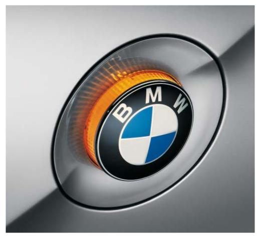
■ Indicator light in front side panel: integrated into the BMW roundel.
