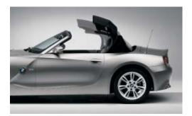
■ Manual softtop operation: central lock for singlehanded operation. (Standard on Z4 2.5i.)
