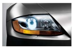
■ Xenon headlights for low and high beam with dynamic headlight range control ensure better illumination of the road ahead and to the side, in bad weather or in poor visibility. Xenon headlights with ellipsoid technology offer a very high standard of light intensity and a very smooth and consistent spread of light on the road.
