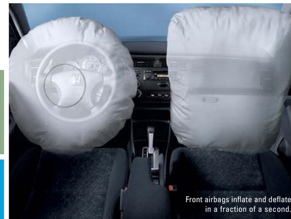
Front airbags inflate and deflate in a fraction of a second.
