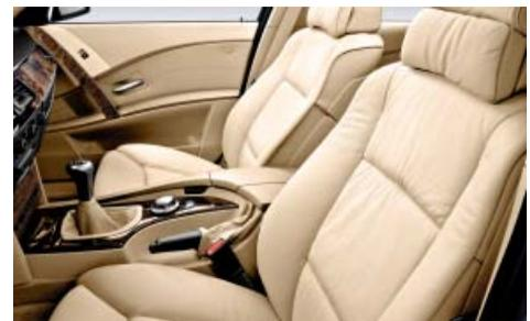
□ **Comfort seats** at the front, electrically adjustable with multi-function control of seat angle, headrest position, backrest angle, seat height and active headrests for the driver and front passenger. Also includes lumbar support, seat depth adjustment, and backrest width adjustment.
