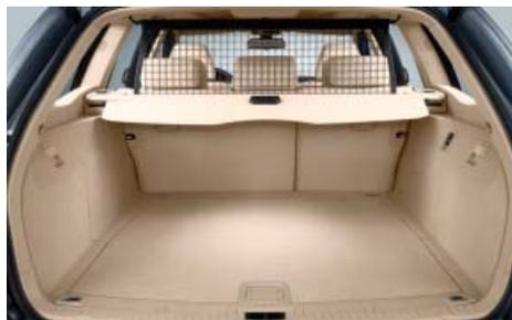
■ **Loading area cover, incl. dividing net:** When the tailgate or rear window is opened, the cover automatically moves out of the way – for easy loading and unloading of the luggage compartment. The dividing net prevents objects from entering the occupant area during hard braking manoeuvres.
