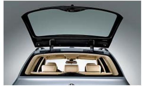
■ **Rear window, with separate opening function:** can be opened separately for quick and easy loading and unloading of objects.
