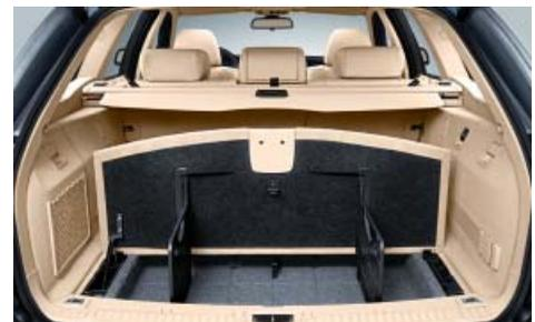
□ **Storage compartment package** for a practical and even more versatile luggage compartment. This equipment package includes an underfloor storage space with adjustable compartments, as well as two foldable dividers for securing objects of different sizes. Also included: straps on the side walls, multi-purpose holders and a net on the left-hand side for smaller items.
