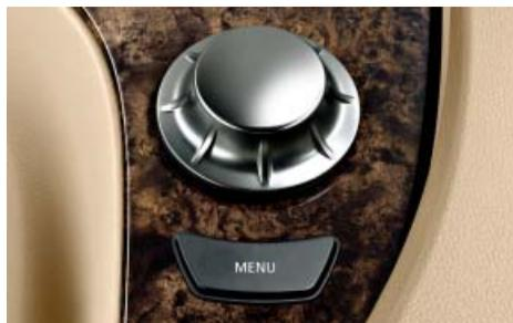
■ **Controller**, the central iDrive control element (for use by driver and front passenger). This turn/press button enables intuitive control of a variety of functions shown on the Control Display. The menu system is based on the four compass directions and provides a choice of four individual menus: climate, communication, navigation and entertainment.
