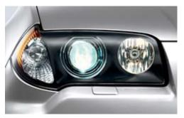
■ Xenon headlights for low and high beam, including automatic headlight range control for much better illumination of the road ahead in bad weather or poor visibility. These headlights also feature auto-levelling to adjust for varying passenger and cargo loads. (Optional on X3 2.5i.)
