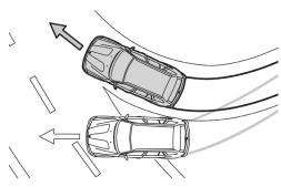
■ Dynamic Stability Control (DSC), comprising ADB-X, CBC, DBC and HDC. DSC detects the risk of swerving right from the start, and stabilizes the car within fractions of a second. The DSC suspension control system ensures greater driving stability, above all in bends.
