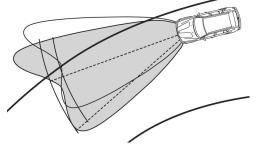
□ Adaptive headlights electromechanically operate the xenon headlights so that they swivel from side to side and thus optimally illuminate a curve the second the driver steers into it, for increased safety when driving at night or when visibility is poor. Sensors register current curve angle, yaw rate and vehicle speed. The headlights then automatically adapt to the determined curve conditions.
