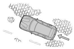
■ Automatic Differential Brake (ADB-X) provides the same function as differential locks by intervening on demand on individual wheels. A wheel about to spin is automatically slowed down by ADB-X until it regains its grip and conveys drive forces. With DSC activated, ADB-X is supplemented by engine output control; without DSC, the function is set to maximum drive and traction.
