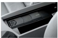
□ **Six-disc CD Changer,** integrated under the armrest. Includes storage compartment for three CDs. The CD Changer can hold up to six CDs and includes an MP3 function.
