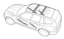
■ Door reinforcements ensure maximum protection in a side-on collision. This safety is provided by diagonal reinforcement profiles in the door, ensuring supreme door stiffness.
