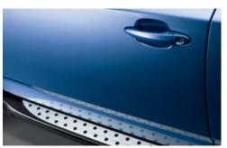
☐ **Running boards** made of brushed aluminum give the X3 a sporty touch and also make entry to the vehicle more comfortable.
