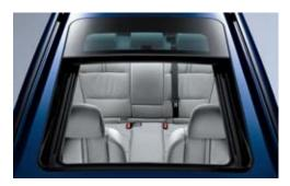
□ Panorama sunroof allows natural light to enter the cabin. For comfort and convenience, it comes with a speed-dependent wind deflector, electric slide and lift control via tip keys, and electric sunshade, as well as trap release and comfort open/close functionality.
