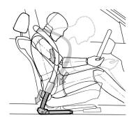
■ BMW restraint system for the driver and front passenger consists of a combination of the three-point seat belt, belt latch tensioner, belt force governor, for optimum restraint in a collision.
