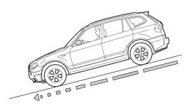
■ Hill Descent Control (HDC) enables your BMW to take even the steepest downhill gradients safely and reliably, automatically reducing the velocity of the car to walking speed without the driver's having to brake. As an option, HDC can also be controlled via buttons in the multi-function steering wheel.
