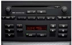
■ Automatic Climate Control system includes Automatic Air Recirculation (AAR), which is activated when a sensor detects certain pollutants in the outside air. Inside, cabin air continuously passes through a microfilter that removes pollen, dust and spores. (Not available on the X3 2.5i.)
