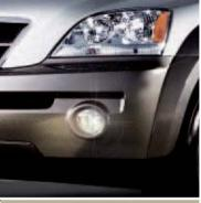
FRONT FOG LIGHTS. A STANDARD FEATURE, FRONT FOG LIGHTS HELP CUT GLARE AND AID VISIBILITY DURING FOG AND INCLEMENT WEATHER. TOGETHER WITH THE SORENTO'S CLEAR-LENS HALOGEN HEADLIGHTS, OUTWARD VISIBILITY AND OVERALL SAFETY ARE GREATLY IMPROVED.
