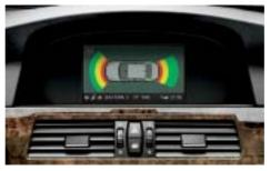
□ Park Distance Control (PDC), front and rear, facilitates parking and manoeuvring in confined spaces; the distance between your car and an obstacle is indicated by an acoustic signal and a visual representation in the Control Display.
