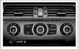
■ Automatic Air Conditioning, with Automatic Air Recirculation (AAR), solar sensor and mist sensor, automatic temperature control and air distribution (separate for driver and front passenger), as well as air quantity control. Also features an air-conditioned storage compartment in the centre console.
