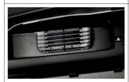
$\Box$  **CD Changer,** for six CDs, integrated into the back of the glovebox.
