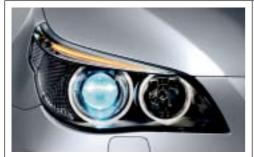
■ Xenon headlights illuminate the road ahead and to the side with brilliant clarity. These headlights also feature auto-levelling to adjust for varying passenger and cargo loads. In conjunction with Adaptive Headlights (optional on the 525i/xi), this also means much improved visibility in bends, as the adjustable headlights are directed into the turn as soon as the vehicle begins cornering.
