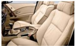
□ Comfort seats at the front, electrically adjustable with multi-function control of seat angle, headrest position, backrest angle, seat height and active headrests for the driver and front passenger. Also includes lumbar support, seat depth adjustment and backrest width adjustment. (Available on the 530i/xi and 550i.)
