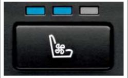
□ **Ventilated seats** for the driver and front passenger. Ventilator fans are built into the outside seats and blow air upwards through an internal web and the micro-perforated Nasca Leather to provide active ventilation. (Available only on the 530i/xi and 550i.)
