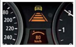
□ Active Cruise Control enables comfortable driving at a pre-set speed. When driving in traffic, your BMW automatically adapts to the speed of a preceding vehicle and maintains a pre-set distance, allowing drivers to concentrate fully on the traffic around them. (Available on the 530i/xi and 550i.)
