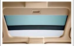
■ Glass sunroof allows natural light to enter the cabin. For convenience, it has a "one touch" open-and-close feature with anti-trapping, as well as a tilt function for ventilating the inside of your car on hot summer days.
