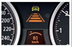
□ Active Cruise Control enables comfortable driving at a pre-set speed. When driving intraffic, your BMW automatically adapts to the speed of a preceding vehicle and maintains a pre-set distance, allowing the driver to concentrate on surrounding traffic.
