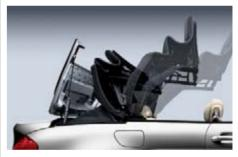
■ Fully automatic softtop operation: the open/close function occurs automatically at the touch of a button (when vehicle is stationary). The vertical rear window can be retracted independently of the softtop. The softtop can also be opened conveniently via the radio remote control.
