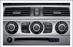
■ Automatic Climate Control with Automatic Air Recirculation (AAR), solar and mist sensors, automatic temperature control and air distribution (separate for driver and passenger), as well as airflow control.
