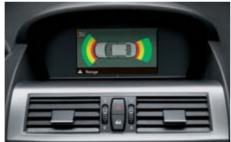
☐ Park Distance Control (PDC), front and rear, uses ultrasonic sensors in the bumpers to help you judge the distance to the car and unseen objects when parking. The system provides both visual and acoustic feedback indicating the proximity of any obstacles.
