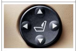
■ Lumbar support is electrically adjustable and provides the driver and front passenger with a high degree of seating comfort and effective spinal relief. The continuously variable air cushion system helps you adopt an orthopaedically correct seating position.
