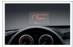
☐ Head-Up Display projects important information such as current speed directly into the driver's field of vision. Direction arrows from the NavigationSystem,ActiveCruiseControlfunctions and Check Control data can also be displayed.
