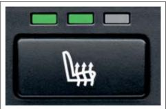
■ Seat heating for the driver and front passenger is a welcome feature in cooler weather. With the touch of a button you can individually select from three heat settings.
