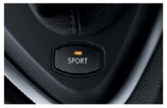
■ Driving Dynamic Control, with Sport Mode, can be activated with the touch of a button. Engine response to the accelerator becomes even more spontaneous and handling is crisper.
