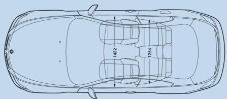
All dimensions of technical drawings in millimetres. Luggage compartment capacity for the M5 is 500 litres and for the M6 Coupé 450 litres (measured to VDA standard).
