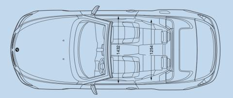
All dimensions of technical drawings in millimetres. Luggage compartment capacity for the BMW M6 Cabriolet is 300-350 litres (measured to VDA standard).
