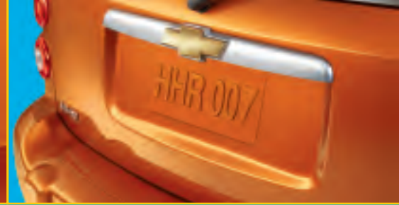
The rear liftgate appliqué features a touchpad latch release.
