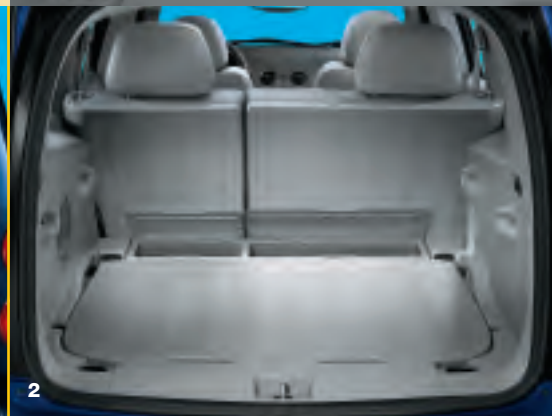
The front-passenger and second-row seatbacks can be folded flat to create an extended loading floor.
