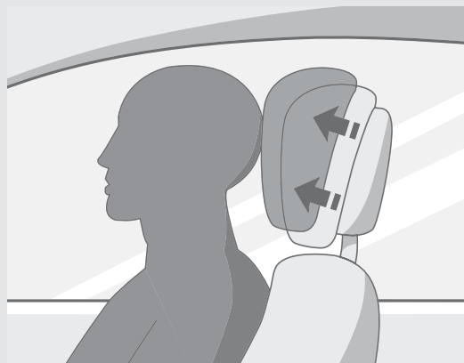
The NECK-PRO head restraints are sensor-controlled.
