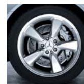
18" 5-spoke light-alloy wheels Front 255/40 R 18 on 8.5J x 18 ET 35 Rear 285/35 R 18 on 9.5J x 18 ET 40 Standard on SL 600
