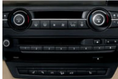
■ **Programmable Memory Keys:** with these buttons, the driver and passenger can save their most frequently used navigation, audio (e.g., certain radio stations or CD tracks) or telephone functions on six separate buttons for rapid access.
