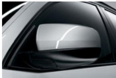
■ **Exterior mirrors, electrically adjustable and heated,** finished in body colour (mirror foot in black), in aspheric design and blue-tinted.
