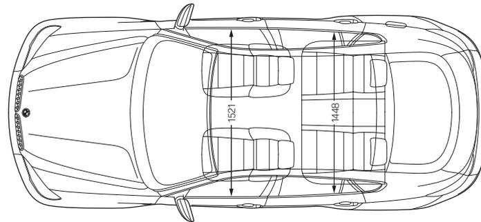
All dimensions of the technical drawings in millimetres. Luggage compartment capacity (VDA method) 570 –1,450 litres.
