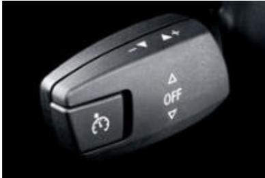
■ **Cruise control with braking function** facilitates comfortable driving at a pre-selected speed.
