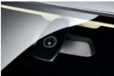
■ **Rain sensor including automatic headlight control:** once activated, the rain sensor automatically switches on the windshield wipers and controls wipe frequency, depending on how hard it is raining. This feature includes automatic headlight control, switching on the low-beam headlights automatically, for example, when it gets dark or when entering a tunnel.
