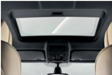
■ **Glass sunroof**, electric, with integral sun protection, comfort opening and closing via vehicle key and fingertip control.
