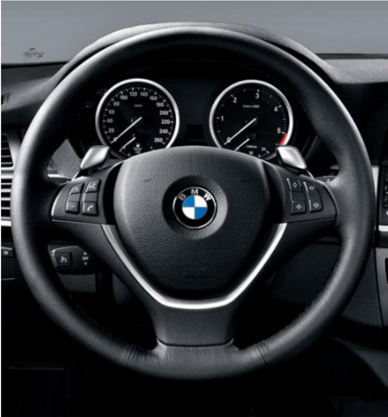
■ **Multi-function leather sport steering wheel**, three-spoke. The buttons on the steering wheel allow for easy operation of audio, telephone, and steering wheel heating functions while keeping your eyes on the road. Two additional buttons which can be programmed to control other functions, such as audio source selection, are also located on the steering wheel.
