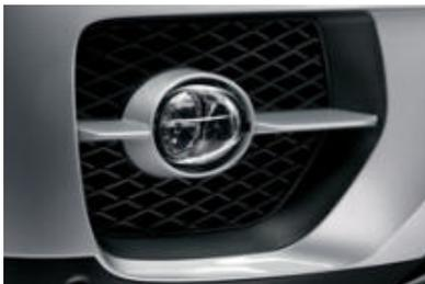
■ **Foglights**, integrated in the front air dam, ensure extra safety in poor visibility. Cornering lights are incorporated into the foglights, providing illumination at an angle of up to 90° to the vehicle when cornering. This allows pedestrians and cyclists to be better seen.
