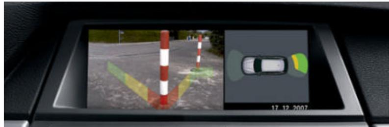
□ **Rear-view Camera** clearly shows the area behind the vehicle on the Control Display, where interactive road line markings show, for example, whether the target parking space is large enough for the vehicle. The Rear-view Camera is activated automatically when the reverse gear is selected.
