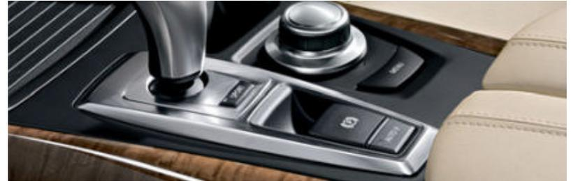
■ **Parking brake with Auto-Hold function,** allows you to hold and release the vehicle most conveniently by means of a button in the central console.
