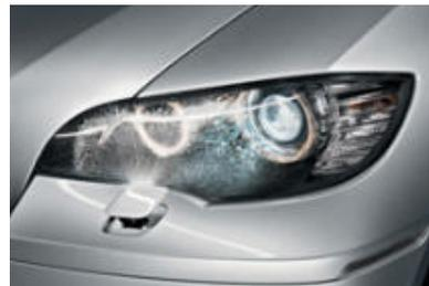
□ **High-Pressure Headlight Cleaning System** provides optimal illumination of the road ahead in all weather conditions. Headlights are automatically cleaned in parallel with the windshield when the lights are on.
