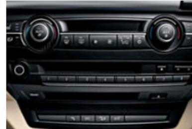
■ **HiFi System** with digital amplifier (205 watt) and 12 loudspeakers, as well as digital equalizing which adapts the sound optimally to the shape of the vehicle interior.
