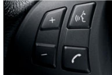
□ **Voice recognition system**, for adjusting e.g., navigation routes while driving. Functions are shown on the Control Display at the same time (this feature is included in the optional Technology Package and is standard on the BMW X6 xDrive50i).
