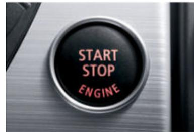
■ **Start/Stop button** for starting the engine. After inserting the ignition key you can start or stop the engine by pressing the button.
