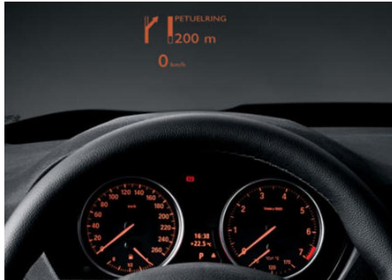
□ **Head-Up Display** projects important travel data, such as current speed, navigation system directions, and cruise control, on the windshield, directly in the driver's field of vision. The height and brightness of the display can be adjusted, so that the driver can fully concentrate on the traffic at all times (optional only on the BMW X6 xDrive50i).
