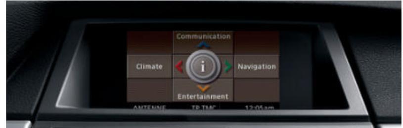
■ **Control Display** with TFT screen (6.5 inch, colour) shows the functions activated by the iDrive Controller (e.g., on-board computer or radio). In conjunction with the Navigation System, the screen measures 8.8 inches.
