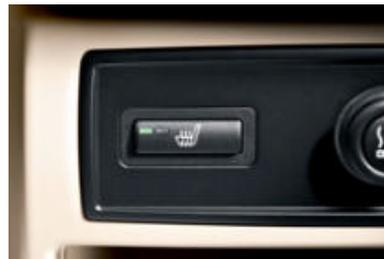
□ **Seat heating at the rear**, with two stages.
