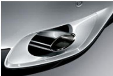
■ **Tailpipes:** The BMW X6 xDrive35i features two circular stainless steel tailpipes with a chrome surround.
