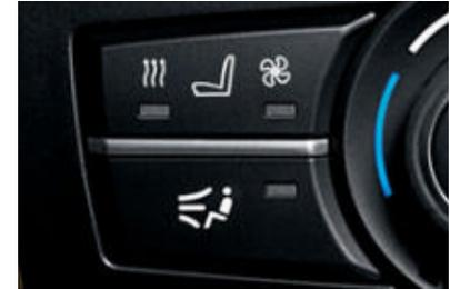
□ **Active seat ventilation** provides a noticeably more comfortable ride. Fans in the seat base and backrest blow air through the seat covers (available for the driver and passenger in conjunction with Nevada Leather, perforated, and Comfort Seats).
