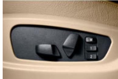
■ **Seat adjustment, electric**, for driver and front passenger, with memory function for driver's seat, steering column, and exterior mirrors.
