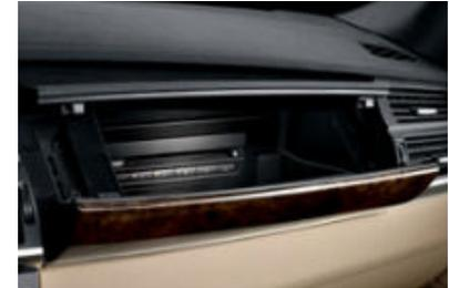
□ **6-disc multi-media changer**, single slot, with features including scan function, random play, and MP3 and DVD audio capability; installed in the glove compartment.
