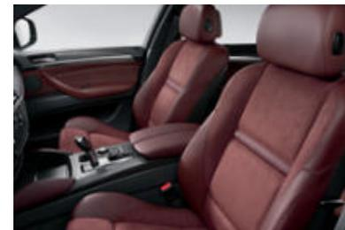
■ **Sport seats** for driver and passenger; highly contoured seat sides for optimal lateral support at all times. Seat height, seat angle, and backrest angle are electrically adjustable; thigh support is manually adjustable.
