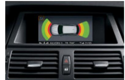
■ **Park Distance Control (PDC)**, front and rear, makes parking easier in the narrowest spaces. The distance between the vehicle and the nearest obstacle is signalled acoustically, as well as visually in the Control Display.
