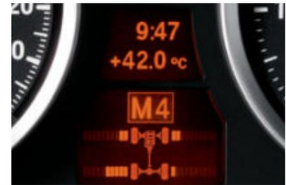
■ **Dynamic Performance Control**: the display in the instrument panel shows how xDrive All-Wheel Drive is distributing drive between the front and rear axle and how Dynamic Performance Control is flexibly distributing power between the rear wheels.
