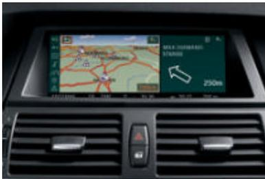
□ **Navigation System** with 8.8-inch colour display: traffic guidance provided by voice information, arrows and street maps. The split-screen function allows you to view radio and navigation data simultaneously.
