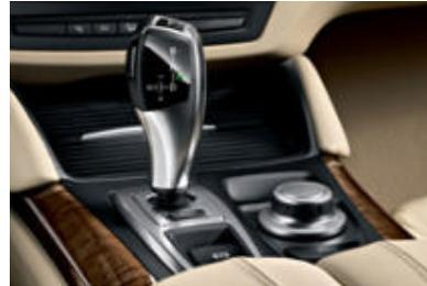
■ **Six-speed Sport automatic transmission with Steptronic®.** Gears are shifted very quickly and smoothly for optimum performance on the road.
