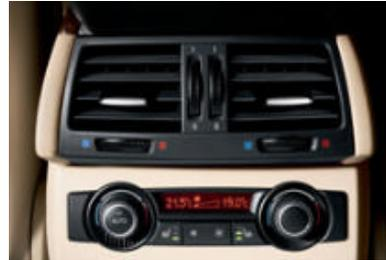
□ **Automatic Climate Control, 4-zone**, provides all the functionality of the 2-zone Climate Control system to passengers seated in the 2nd row. Two dials and a display at the back of the centre console allow for easy control. Additional air outlets and footspace heaters are also included.
