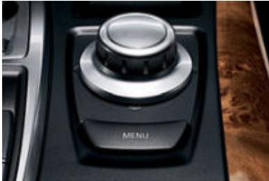
■ **Controller** is the central iDrive input element (for driver and passenger). Additional functions can be activated from the control display using this rotary/push button. Menu navigation is oriented to the four cardinal points. Different menus are available: Climate, Communication, Navigation, Entertainment, and on-board information.
