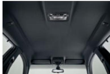
□ **Anthracite roofliner**: the A-, B-, C- and D-pillar trim, as well as the sun visors and roof grab handles, are finished in refined Black (included in Sport Packages).
