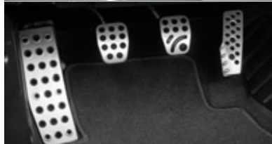
FOOT REST — ALUMINUM PEDAL (ACCELERATOR) — ALUMINUM PEDAL (BRAKE) — ALUMINUM (A/T) PEDAL (BRAKE AND CLUTCH) — ALUMINUM (M/T)
