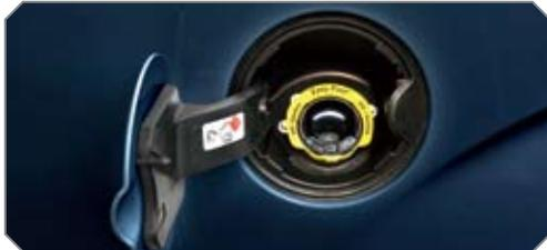
**New Easy Fuel™ Capless Fuel Filler** is standard on F-150. It eliminates the fuel cap, so you don't have to remove it or remember to replace it, and it creates a positive seal for the fuel port. Just open the fuel door, gas up, close the door and go. How easy is that?
