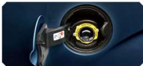
**New Easy Fuel™ Capless Fuel Filler** is standard on F-150. It eliminates the fuel cap, so you don't have to remove it or remember to replace it, and it creates a positive seal for the fuel port. Just open the fuel door, gas up, close the door and go. How easy is that?
