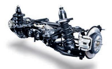
Unlike the solid rear axle on most trucks, the Ridgeline has front and rear independent suspension. So its rugged off-road abilities are paired with a refined on-road ride, a stable, firmly planted feel, responsive steering and confidence-inspiring cornering. And you still get more than 208 mm (8 inches) of ground clearance.
