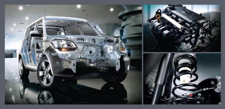
RIGID BODY STRUCTURE is designed to absorb crash energy and direct it away from the occupants inside Soul's strong and protective passenger compartment. QUICK AND RESPONSIVE POWER comes from a choice of two DOHC four-cylinder engines – a fuel-efficient 1.6-litre engine and an available 2.0-litre engine with 142 horsepower. And they both feature performance-enhancing continuously variable valve timing (CVVT).
