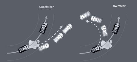
ELECTRONIC STABILITY CONTROL automatically adjusts brake pressure at the appropriate wheel or wheels and regulates engine torgue to correct Soul's path. It's standard on all Soul 2.0L models
