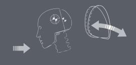
ANTI-WHIPLASH FRONT HEADRESTS move forward and upward in the first milliseconds of a crash to help reduce neck injuries.
