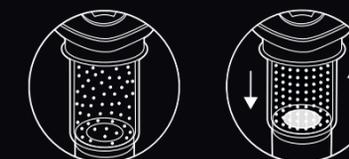
CTS-V's Magnetic Ride Control suspension is so advanced, it can adjust the damping of the individual shock absorbers up to 1000 times per second to provide precisely the right balance of handling agility and body control.
