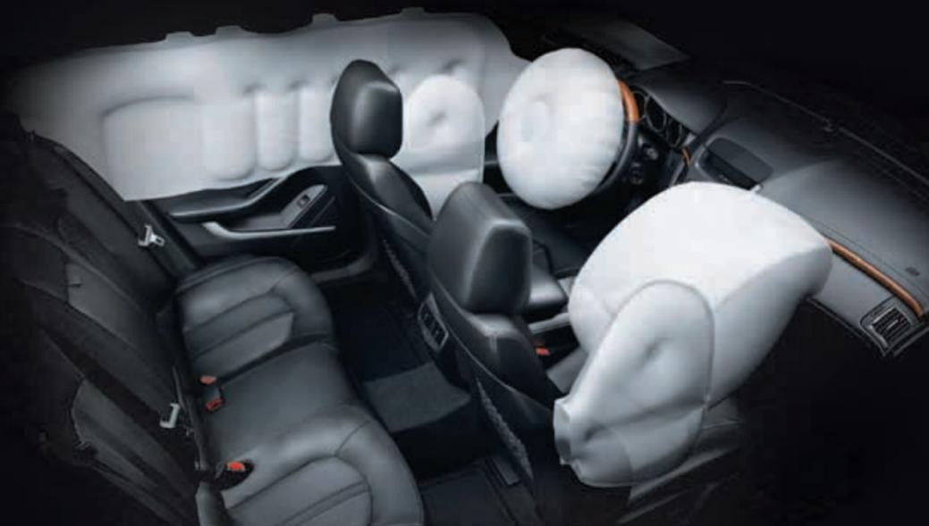
In the event of a crash, CTS is equipped to help protect you with dual frontal air bags, seat-mounted side-impact air bags and front-to-rear roof-mounted side curtain air bags.\*\*
