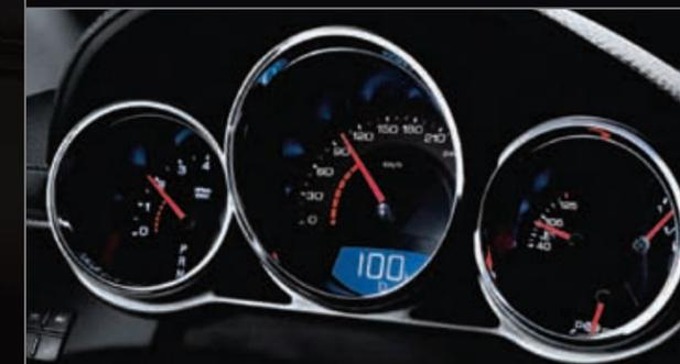
To signal the need for an up-shift, the LED tracers around CTS-V's tachometer begin to flash as the supercharged 6.2L V8 approaches redline.
