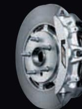
With very massive ventilated discs at all 4 wheels, 6-piston calipers in the front and 4-piston calipers in the rear, CTS-V's Brembo braking system provides tremendous stopping power, even after a series of hard stops from high speeds.
