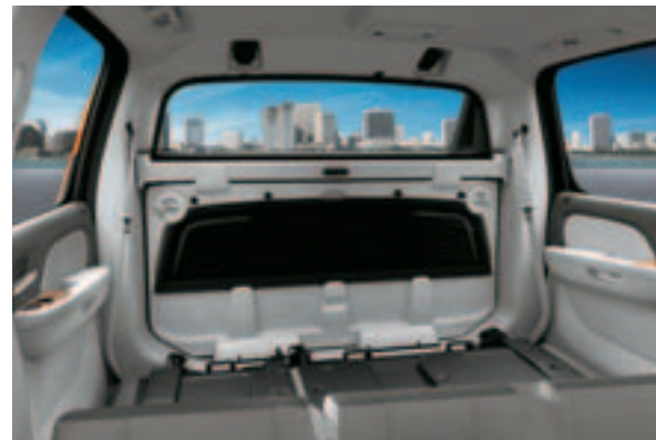
Folding down the split rear seat increases cargo capacity and initiates the easy conversion of the cabin from SUV to pickup.
