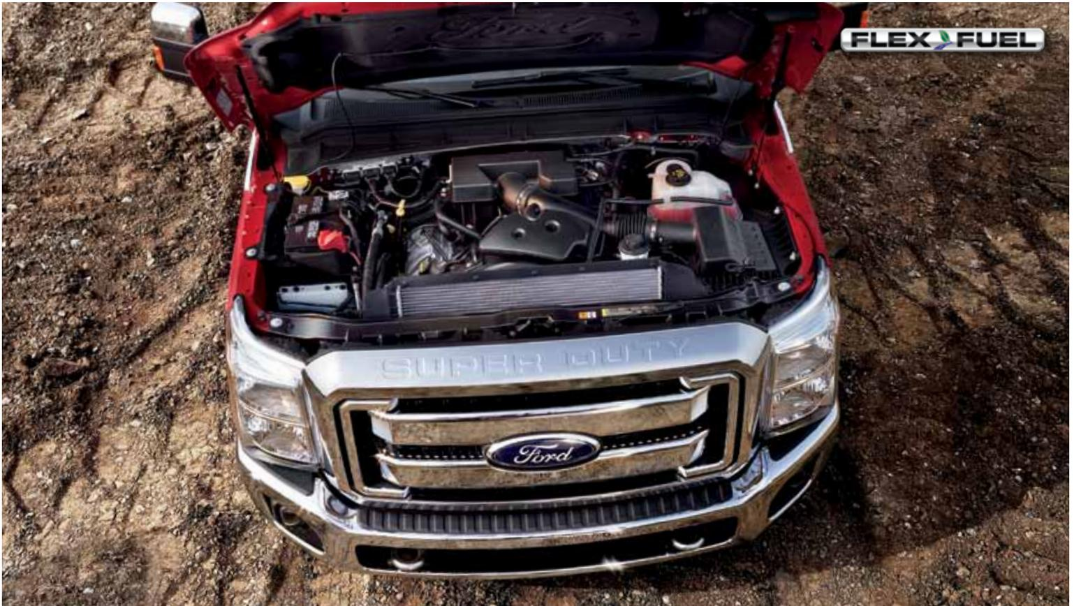
**Produces significant low-rpm torque.** The stiff SOHC valvetrain with roller-rocker shafts also enables an intake- and exhaust-port layout that optimizes airflow.
