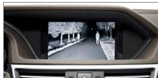
Utilizing radar technology, Night view assist provides a clear view of the road ahead when driving at night or in dark conditions.
