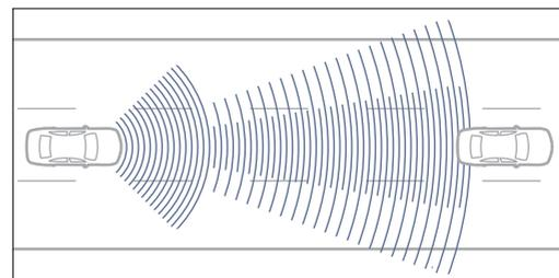
DISTRONIC PLUS reduces the chance of rear end collisions by automatically braking in the event of danger.
