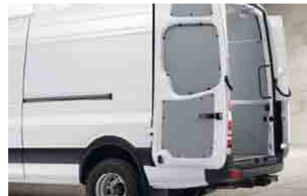
Hinged rear doors which open up to the side wall (and lock into position automatically) are available as standard equipment
