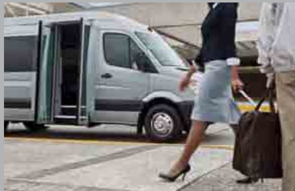
Wide .97 meter (38 inches) outward opening side doors and low step-in for quick and easy loading of up to 18 people
