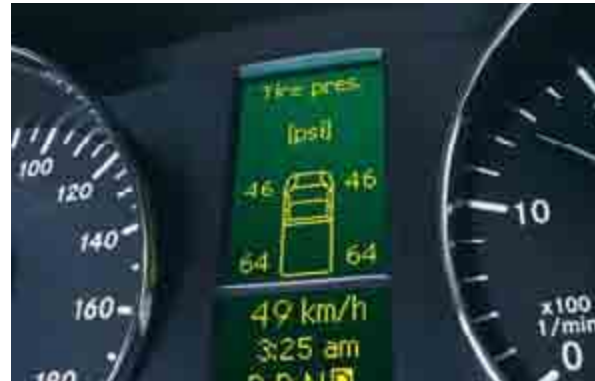
Tire pressure monitoring system (standard for Cargo Van and Passenger Van; not available in conjunction with Cab Chassis or twin tires)
