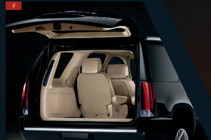
2 The standard power liftgate can be opened or closed by pressing a button on the key fob. Additional switches are located on the instrument panel and in the cargo area.
