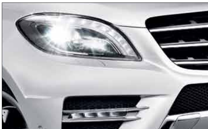
Bi-Xenon headlamps with LED daytime running lights.
