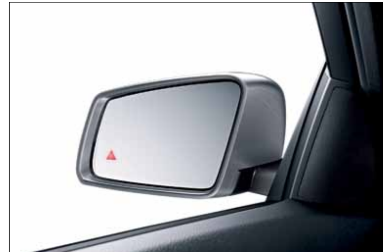
Passive Blind Spot Assist alerts the driver if it identifies a risk of a collision while the vehicle is changing lanes.
