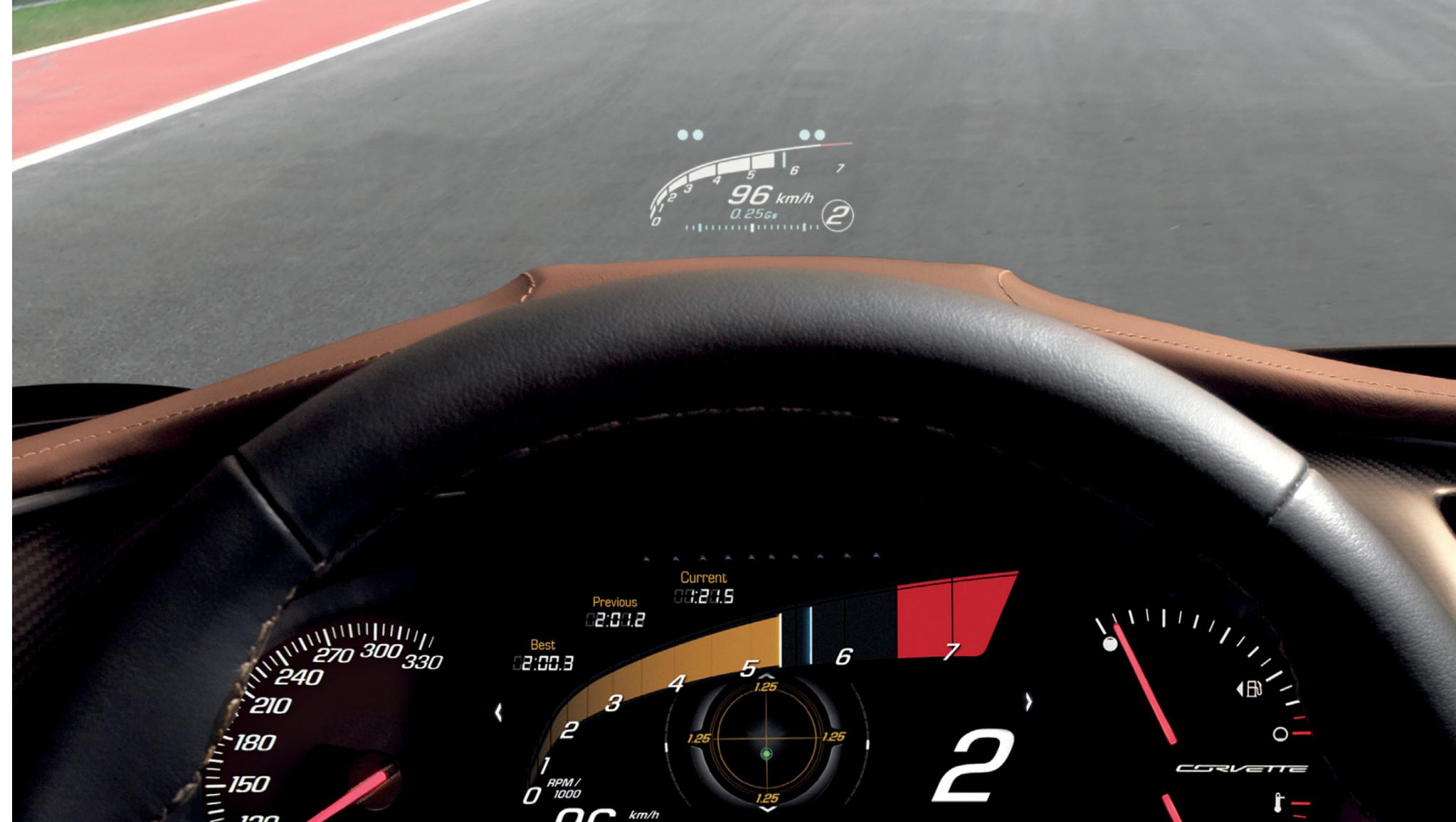
**PERFORMANCE TRACTION MANAGEMENT.** With this system (included and only available with Magnetic Ride Control), five separate settings of torque reduction and brake intervention facilitate maximum grip on the road for more confident driving.
