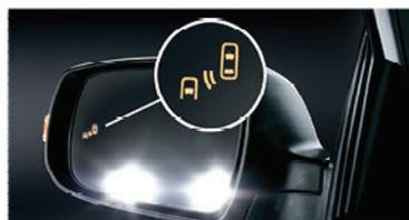
**BLIND SPOT DETECTION (BSD).<sup>1</sup>** BSD uses radar sensors in the rear bumper of the vehicle to detect vehicles you may not be able to see because they're in your "blind spot". When the system identifies a vehicle in a blind spot, it activates a warning light in the side mirror to warn you. If the vehicle is present when you signal for a lane change, an audible alarm sounds to help you avoid a possible collision. Standard on Sorento SX.
