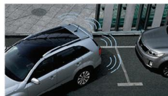
**BACK-UP WARNING SYSTEM.<sup>1</sup>** Using rear bumper-mounted sonar sensors, this standard system alerts you to potential obstacles behind the vehicle when you're backing up.
