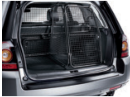
Cargo Barrier with Divider Separates pets from cargo and has a lockable outer gate on one side. Cargo divider can also be used with cargo barrier – half height.
