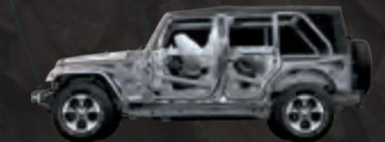
**SPORT BAR** High-strength steel is integrated into the B-pillar that runs into the floor, helping to improve side-impact performance and vehicle stiffness on every Wrangler.
