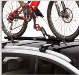
Roof-mounted bike rack
