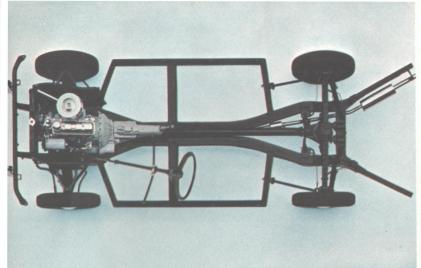
Four-wheel independent suspension stabilized by a torsion bar levels any road at any speed. You'd usually associate this sports car suspension and heavy channel-steel frame with far more expensive cars.
