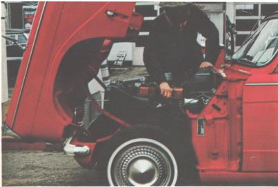
Single hood and fender unit tilts forward for easy access. American tools fit every part. Only four parts need lubrication (every 3,000 miles) because nearly all metal parts are nylon or rubber lined.
