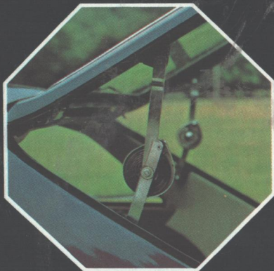
Counter-balanced rear door for one hand operation. The optional, electrically heated rear window stays mist free.
