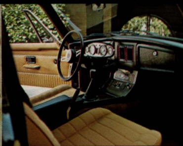
Interior: corded brushed nylon reclining bucket seats, complete instrumentation, lockable glove box and center console.
